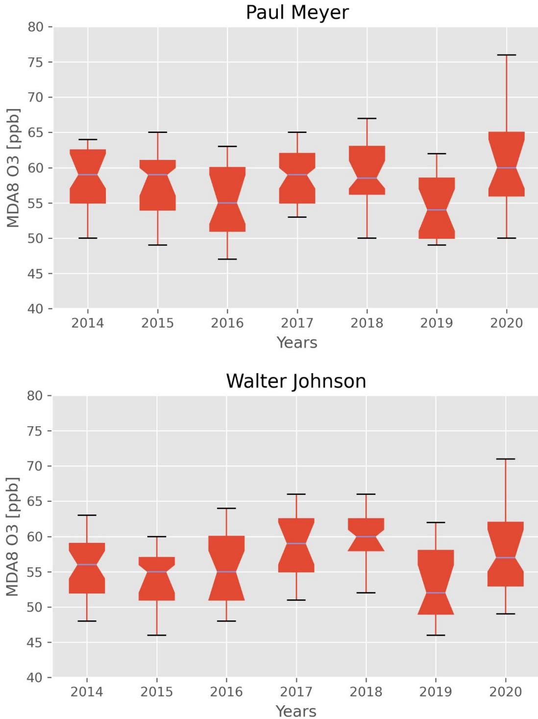
Figure G-2. Annual May distributions of MDA8 ozone at sites with exceptional events during May 2020. Notches denote 95th confidence interval of the median, boxes are 25th, 50th and 75th percentiles, and whiskers are 5th and 95th percentiles.
